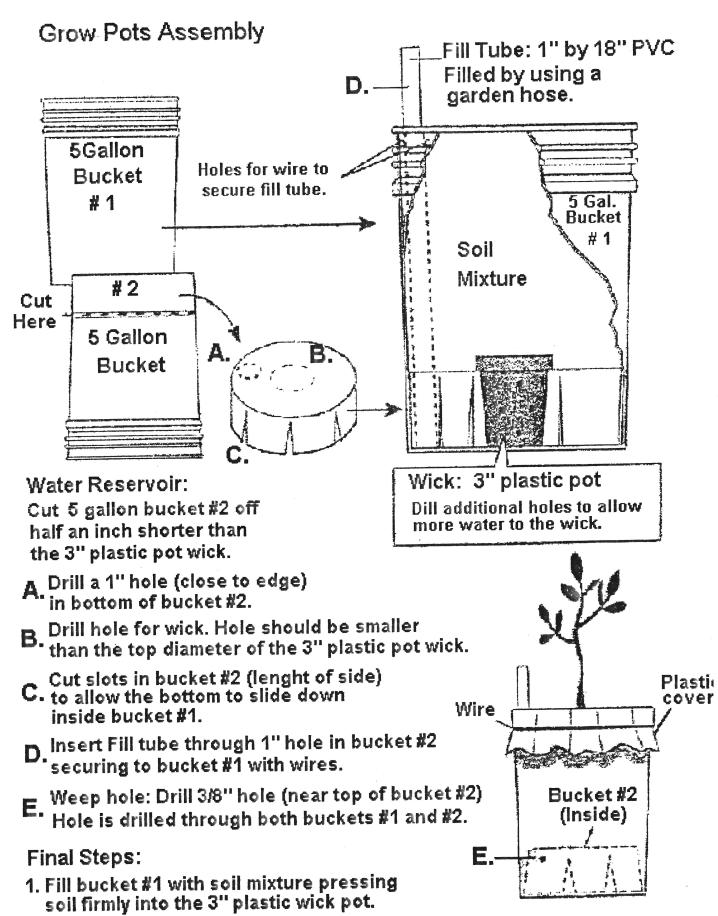
2. Secure plastic cover with wire. Cut an X in middle of the plastic and insert a plant.
