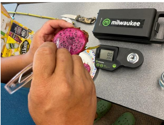
Using the Brix meter to check the sweetness level of the fruit.
